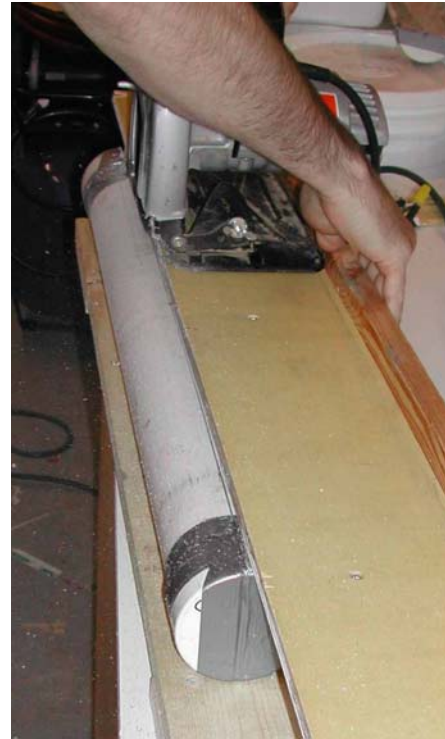
Fig. 9. Core tubes were opened lengthwise by circular saw. A custom-made holder held the tube firmly and served as a guide for the saw so that the blade moved along the tube at the correct position.
