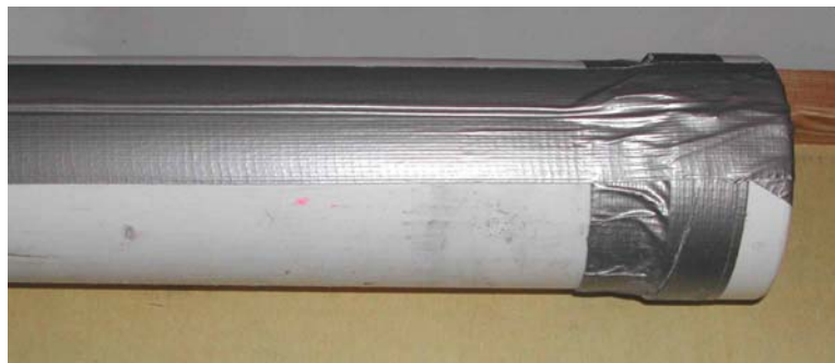
Fig. 10. The first lengthwise cut on the core tube was taped with duct tape to prevent loss of material while the second cut was made on the opposite side of the tube
