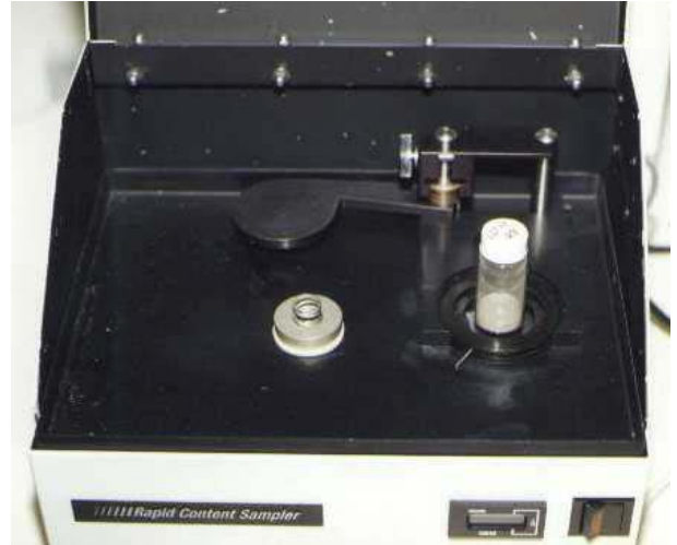
Fig. 18. The Rapid Content Sampler is open showing a dry sample in a scintillation vial in place for scanning through the quartz window (right). A mechanical iris is used to position the vial in the centre of the window. The external ceramic reference is in the centre of the photo
