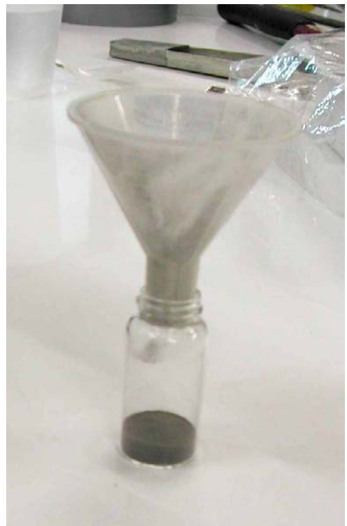
Fig. 13. The dried samples were pulverized using a mortar and pestle and placed in glass scintillation vials for scanning in the dry state and subsequent chemical analysis
