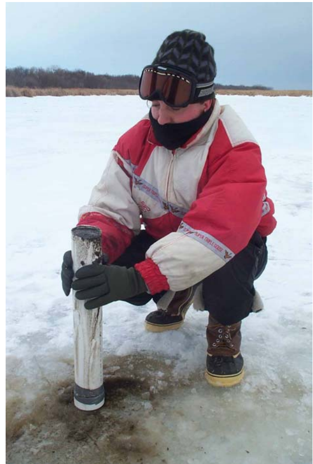
Fig. 6. Core tube sawn off at the top of the sediment ready to be capped for transport
