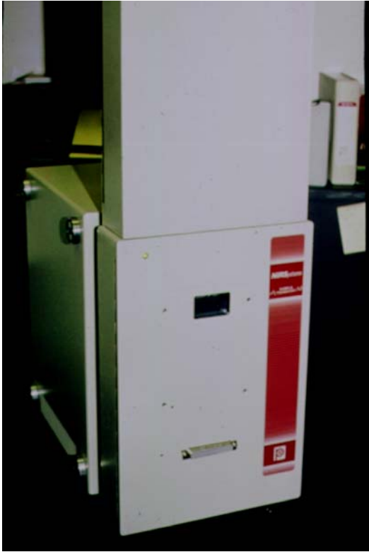
Fig. 14. Foss NIRSystems model 6500 scanning spectrophotometer fitted with standard transport. The sample cell in Fig. 15 fits into a holder in upper part of the sample transport. The cell moves to the lower part of the sample transport for scanning.
