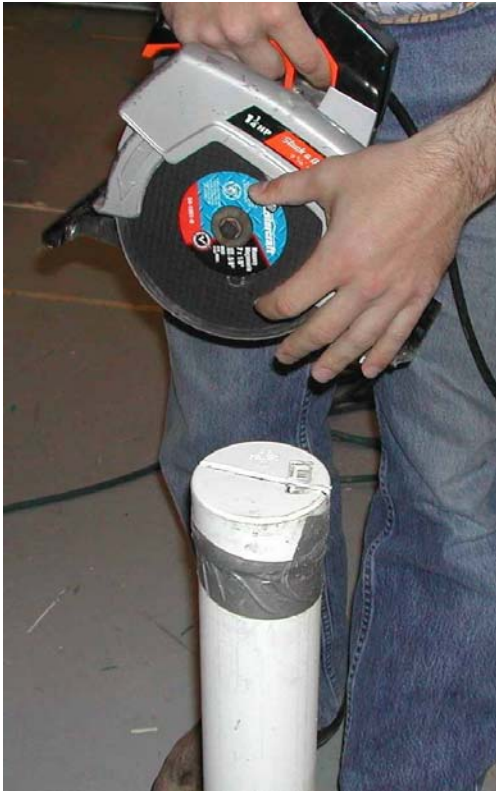
Fig. 8. The ends of the core tubes were sawn with a circular saw. The opening was sealed with duct tape.
