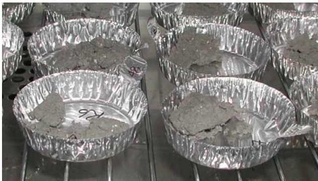
Fig. 12. After scanning on the NIR instruments each slice was divided into two portions and oven-dried to constant weight
