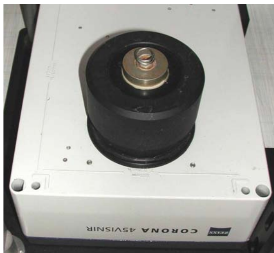
Fig. 22. External ceramic reference in place on the Corona sensor head
