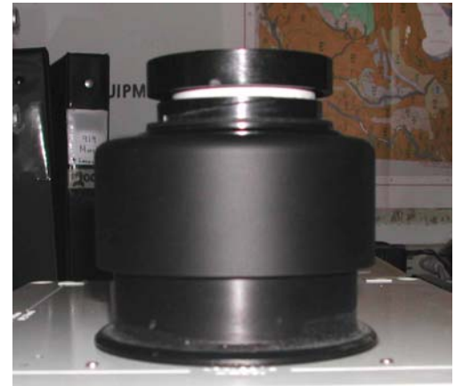
Fig. 20. The Zeiss Corona scanning the white reference inside a Foss standard sample cell. The reference was scanned between each sample. The samples were presented in the standard sample cell as in Fig. 15.
