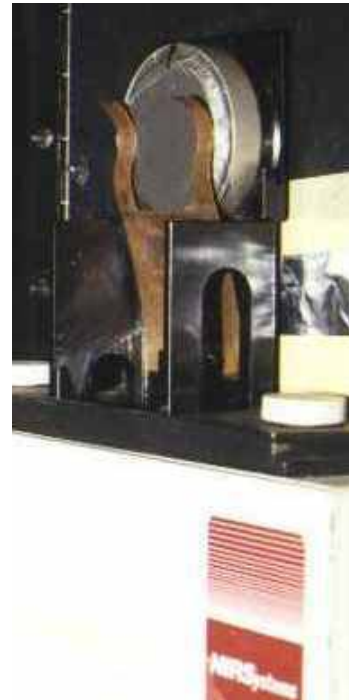
Fig. 16. The sample holder in the upper module of the 6500 with a sample cell in place
