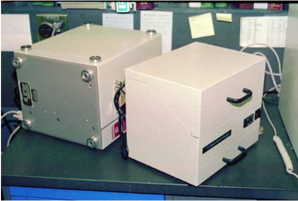
Fig. 17. The 6500 instrument (back) is turned on its side and connected to the Rapid Content Sampler (front) that is closed.
