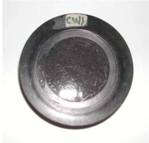
Fig. 15. The standard sample cell, 7.4 cm o.d. used to scan the field-moist samples in the 6500 and Corona NIR instruments. The quartz window is 5.0 cm in diameter. The cell is shown here filled with a field-moist sample.
