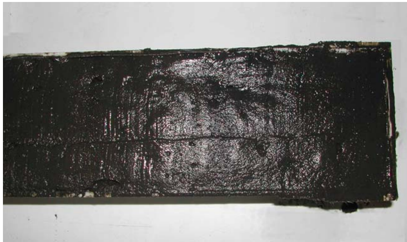
Fig. 11. The core in one half of the core tube completely filled the length of the tube. The material was generally consolidated, except for the first one of two cm at the top that were a thick slurry.
