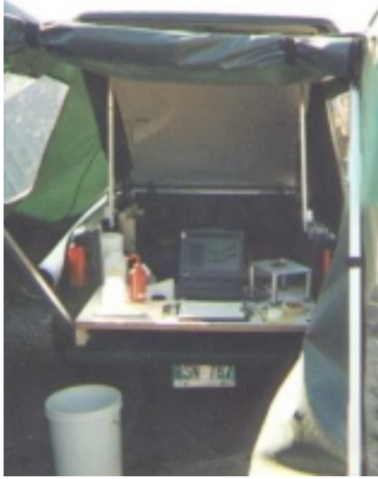
Fig. 5. Moveable lab bench (see Table 3) slides back over tailgate for operation
