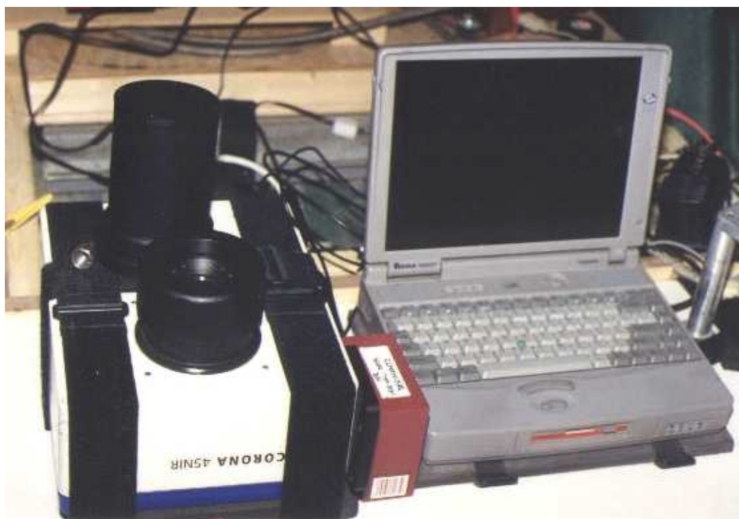
Fig. 1. The Corona® fastened to the bench of the truck lab with Velcro straps with the head, containing the light source and the polychromator (sensors) facing upwards. It was powered by 600-amp/hour bank of batteries and operated from the notebook computer using Aspect Plus software. The black tower for obtaining the dark reference (noise) is behind the head.
